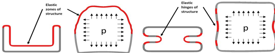
Fig. 5. Deployment of components with flexible areas hinges
