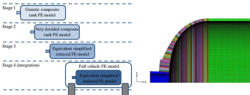
Fig. 8. Stages of CNG tank modelling and detail of stage 1 model
