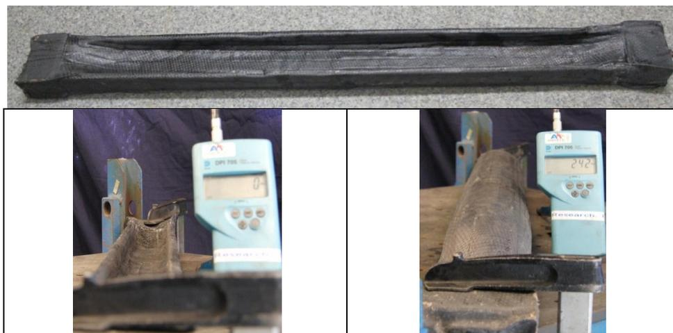
Fig. 2. Expansion of generic expandable fibre reinforced plastic beam
