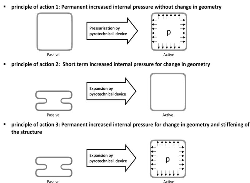
Fig. 4. Pressurisation of components
