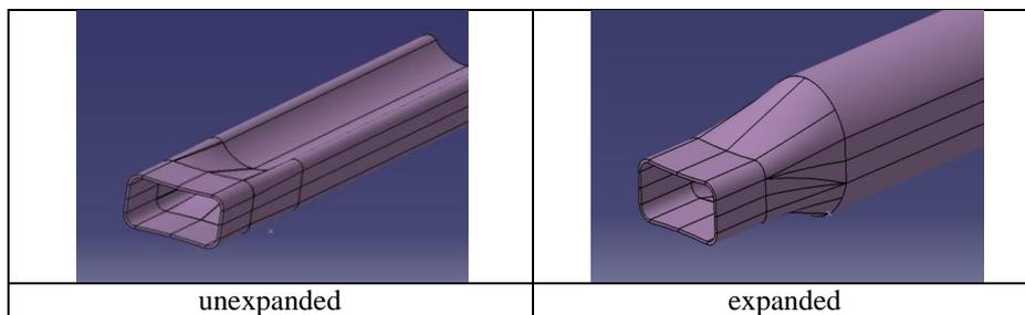
Fig. 1. Geometry of generic active beam
