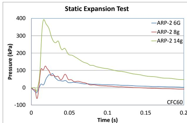
Fig. 3. Pressure of gasgenerators
